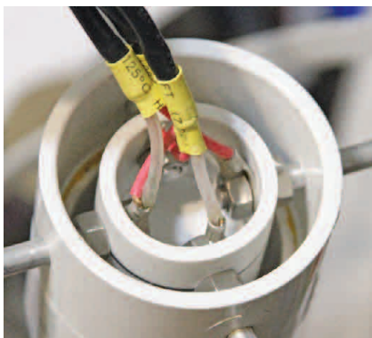
Figure 6 — Feed-point connections.
