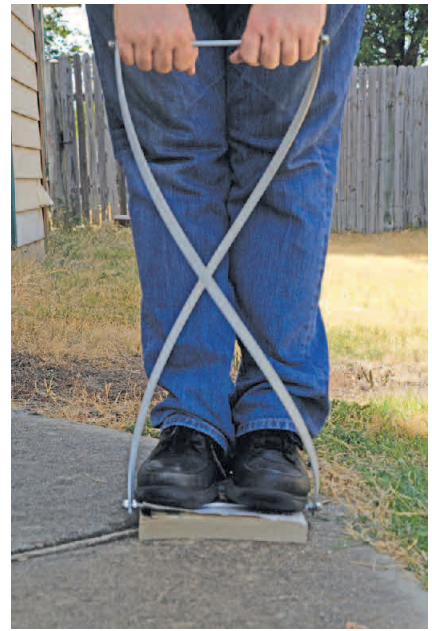
Figure 3 — Hold one aluminum rod end of the rectangle in your hands while standing on the other end of the rectangle on top of the book, and twist the rectangle to the right while pushing down.
